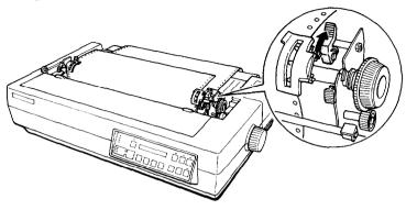
10. Attach the paper guide and lower it so that it is resting on top of the printer. Center both edge guides.
